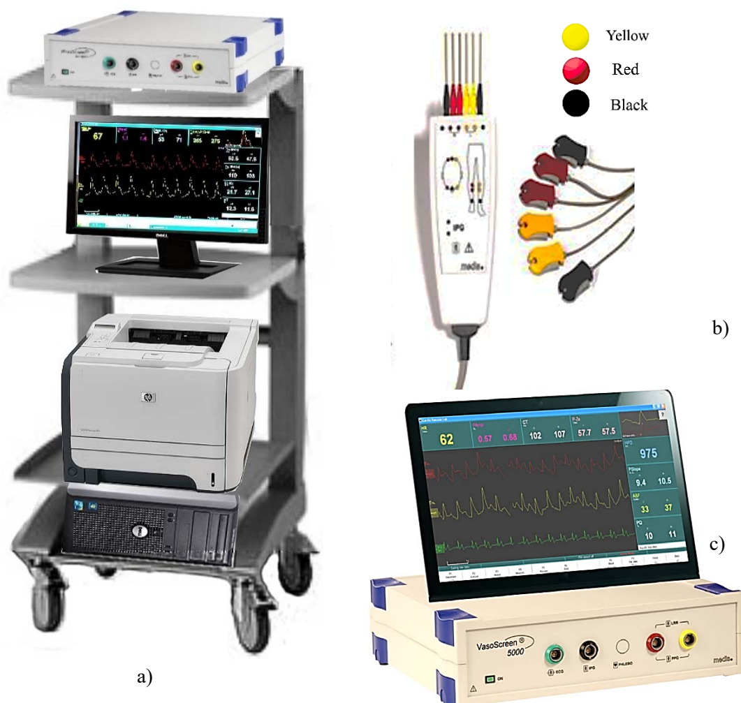
Figure 1. Types of equipment used for measuring rheography. (a) Input and output of the monitoring device, (b) System of electrodes, and (c) VasoScreen 5000 device.
